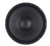
The new B&C 18RBX100 anchors our ferrite subwoofer line, and features an all new FEA optimized motor structure. The 25mm high, 4" (100mm) diameter copper wire voice coil is combined with a laminated double silicone spider, water resistant curvilinear cone and triple roll surround, for even more excursion and linearity.
